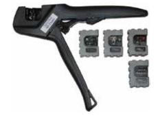
The Draka QuickCrimp handles a wide range of crimping applications. Interchangeable dies enable the user to tackle wire sizes from 26 to 8 AWG with one tool. Ergonomic design provides comfort while rugged construction delivers durability.
